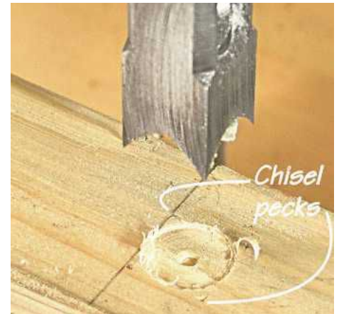
▲ Pic.7 'Touching on' revealed that the chisel was unfortunately slightly off the pencil line
